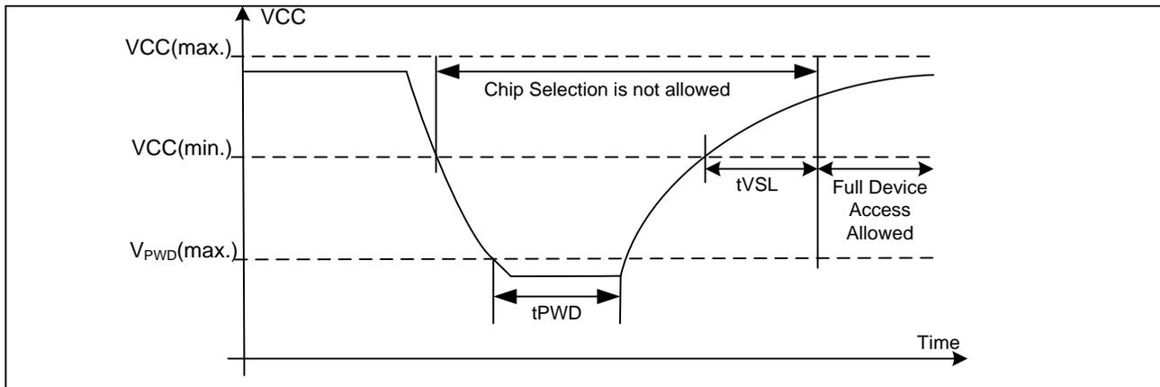
Table 3. Power-Up Timing and Write Inhibit Threshold
