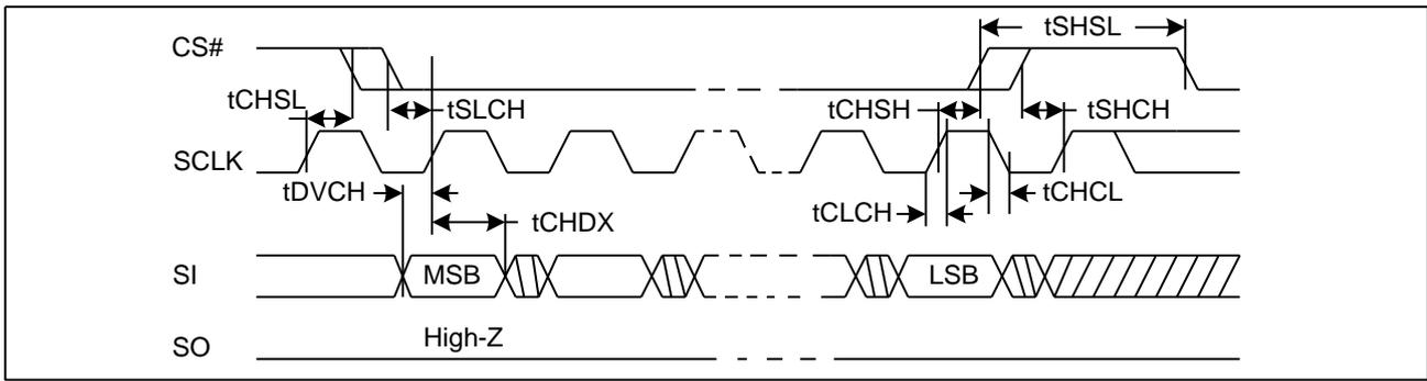
Figure23. Output Timing
