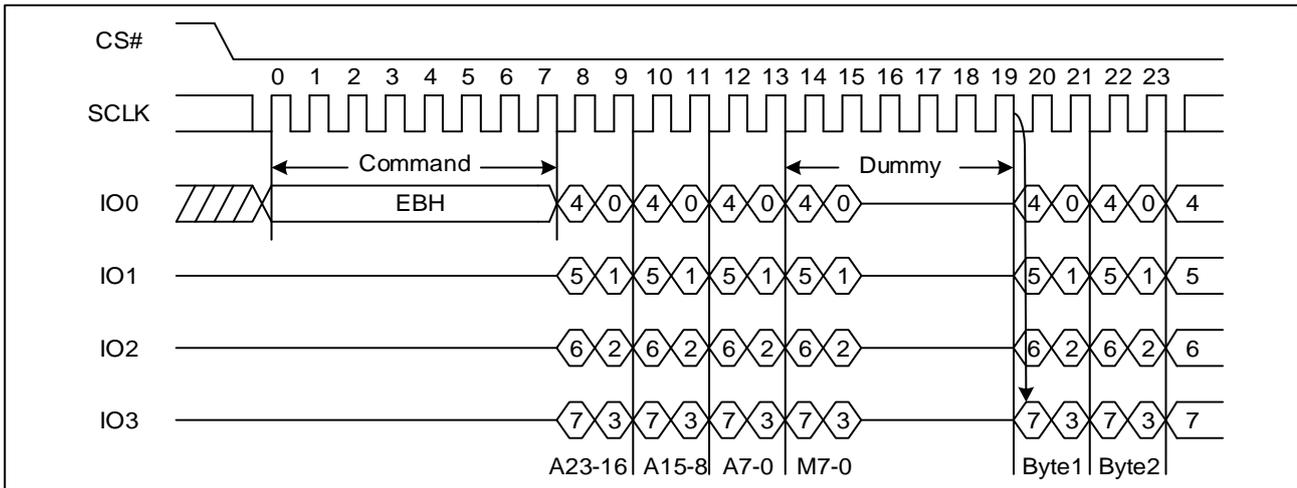
**Figure 14. Quad I/O Fast Read Sequence Diagram ((M5-4) = (1, 0))**
