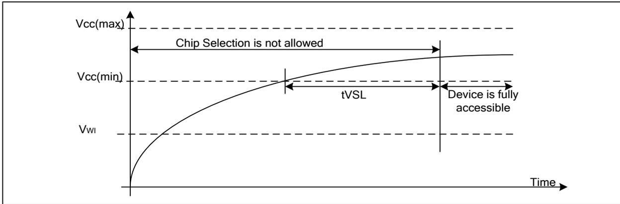
Table 20 Power-Up Timing and Write Inhibit Threshold
