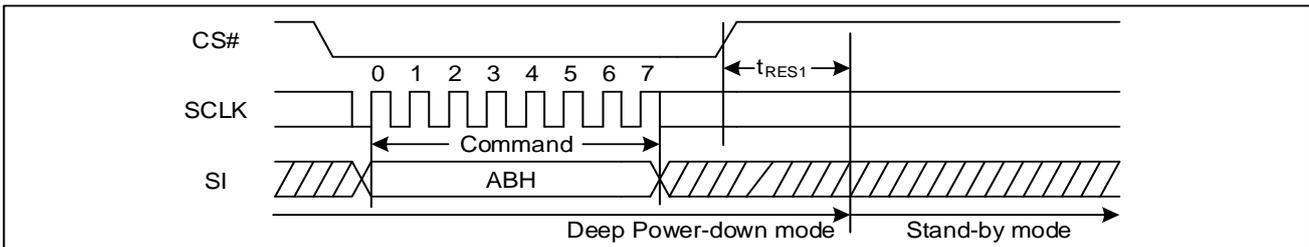
Figure 65 Release Power-Down Sequence Diagram (QPI)
