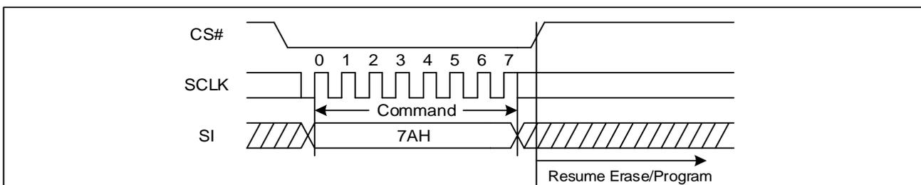
**Figure 76 Program/Erase Resume Sequence Diagram (QPI)**
