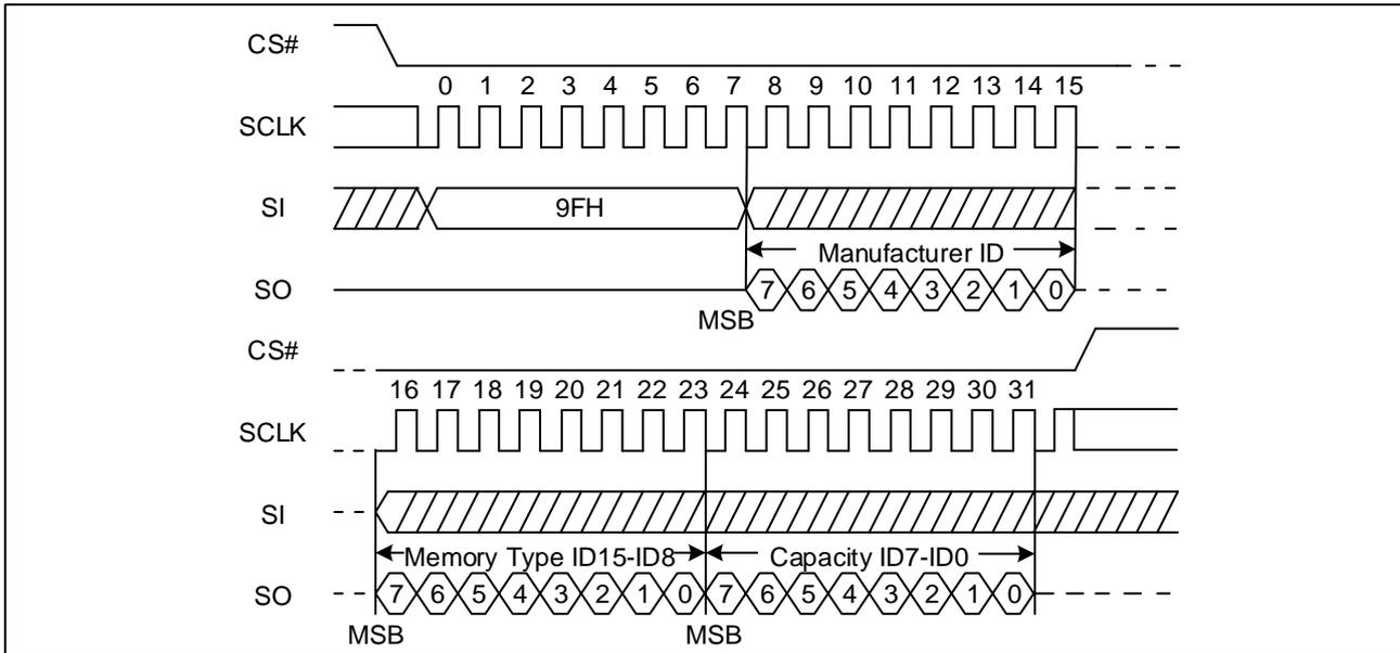
**Figure 72 Read Identification ID Sequence Diagram (QPI)**
