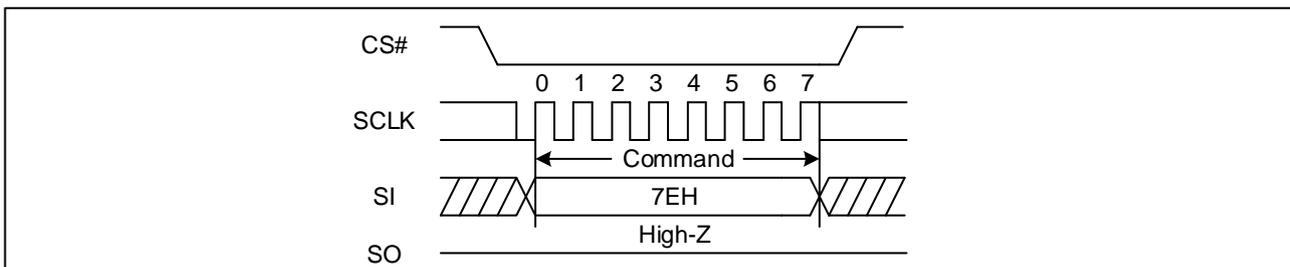
Figure 81 Global Block/Sector Lock Sequence Diagram (QPI)
