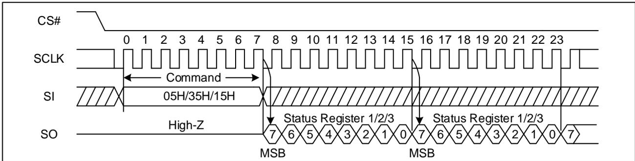
**Figure 28 Read Status Register Sequence Diagram (QPI)**
