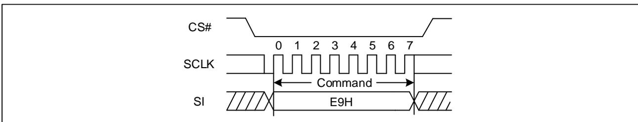
Figure 10 Disable 4-Byte Mode Sequence Diagram (QPI)
