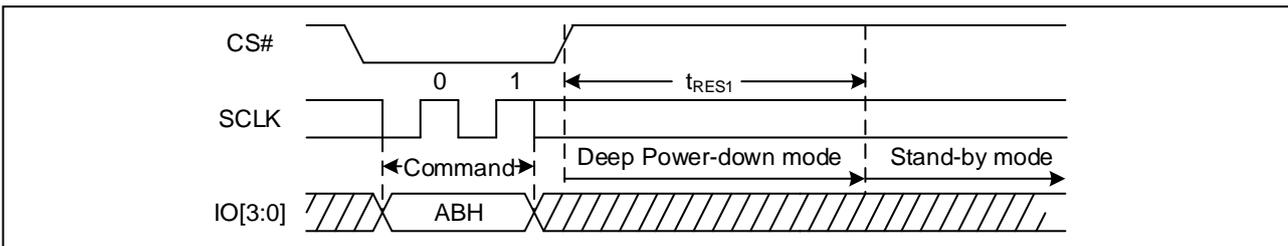
Figure 66. Release Power-Down/Read Device ID Sequence Diagram (SPI)
