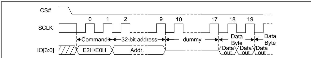
Note: The Read NL Register (E2h) / VL Register (E0h) command uses only 32-bit address input in either 3-Byte or 4-Byte Address mode.
