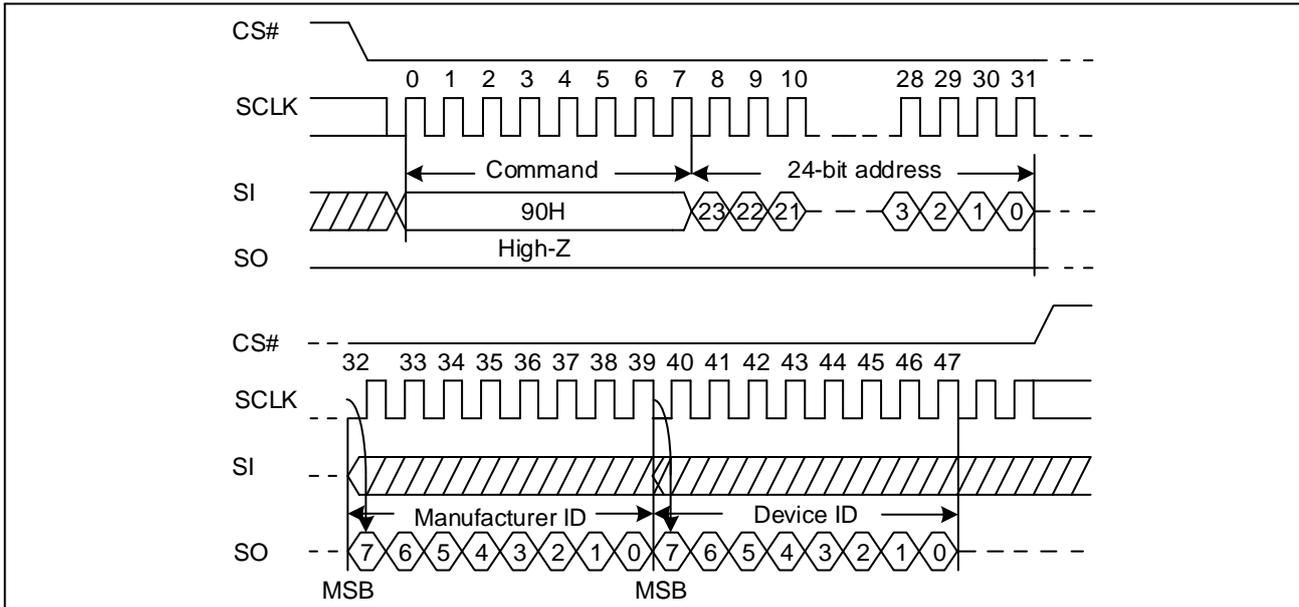
**Figure 70. Read Manufacture ID/ Device ID Sequence Diagram (QPI)**
