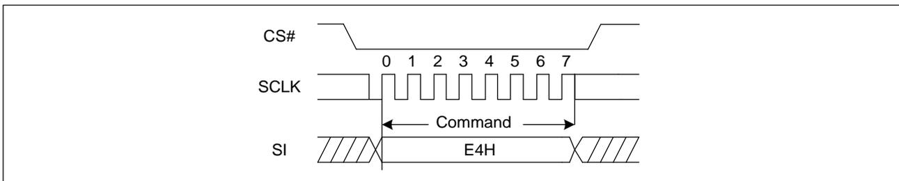
**Figure 87 Clear All NL Registers Sequence Diagram (QPI)**
