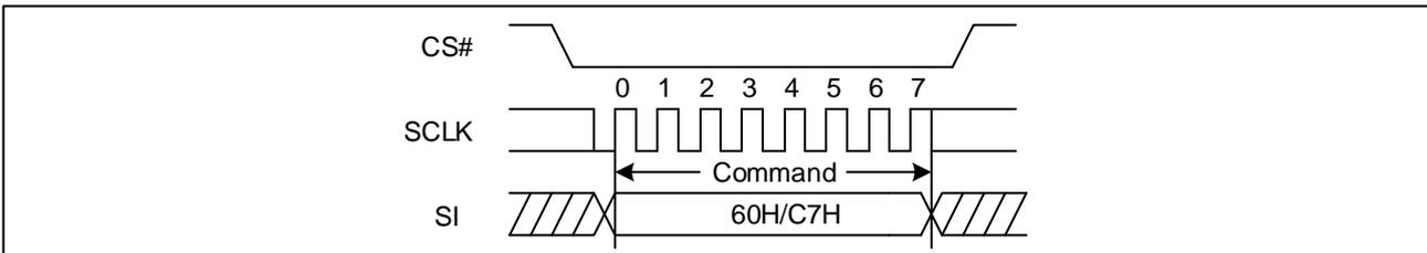
**Figure 59 Chip Erase Sequence Diagram (QPI)**
