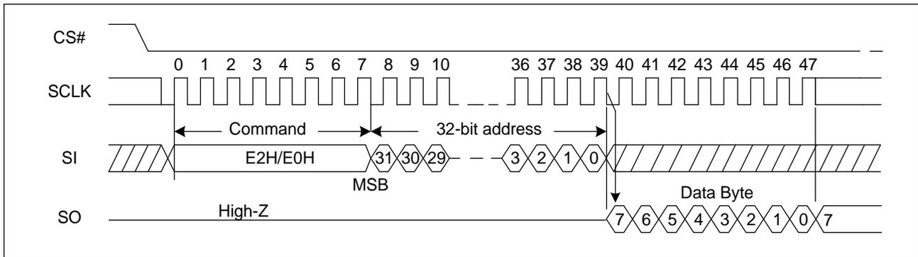
Note: The Read NL Register (E2h) / VL Register (E0h) command uses only 32-bit address input in either 3-Byte or 4-Byte Address mode.
