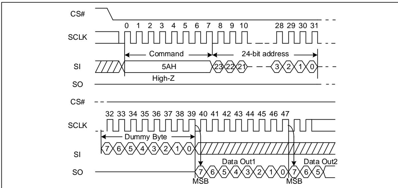
**Figure 95 Read Serial Flash Discoverable Parameter command Sequence Diagram (QPI)**
