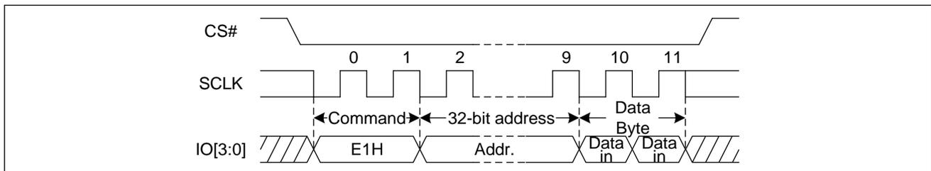
Note: The Write VL Register command uses only 32-bit address input in either 3-Byte or 4-Byte Address mode.
