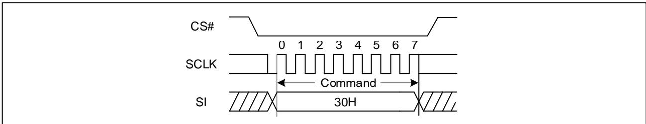
**Figure 12. Clear Status Register Flags Diagram (QPI)**
