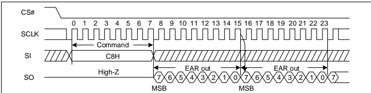
**Figure 34 Read Extended Address Register Sequence Diagram (QPI)**
