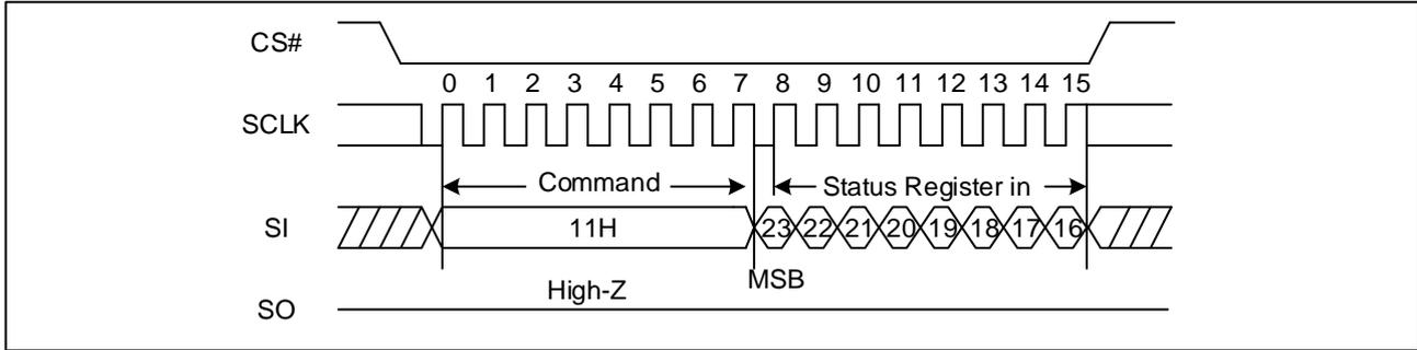
**Figure 22. Write Status Register-3 Sequence Diagram (QPI)**
