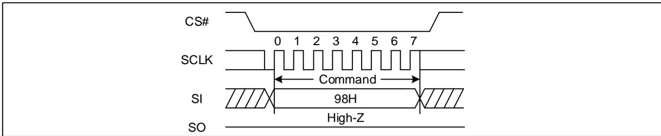
**Figure 83 Global Block/Sector Unlock Sequence Diagram (QPI)**
