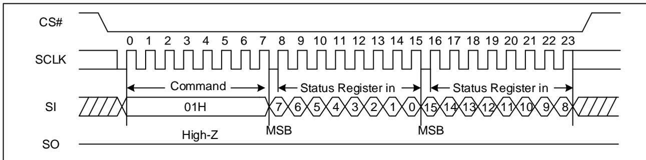
Figure 20. Write Status Register-1&2 Sequence Diagram (QPI)
