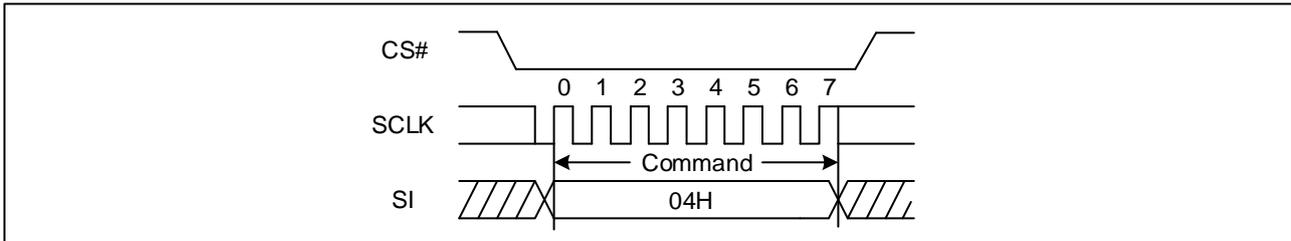
**Figure 16 Write Disable Sequence Diagram (QPI)**
