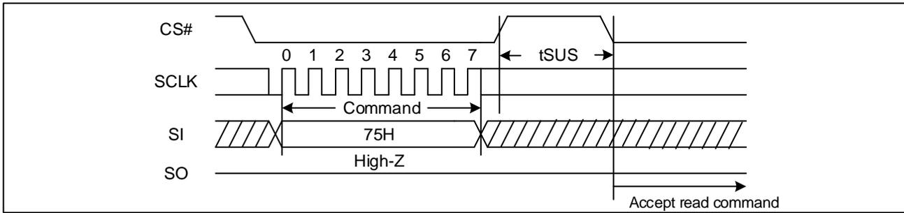
**Figure 74 Program/Erase Suspend Sequence Diagram (QPI)**
