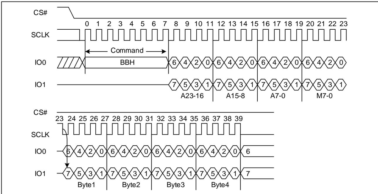
**Figure 14. Dual I/O Fast Read Sequence Diagram ((M5-4) = (1, 0))**
