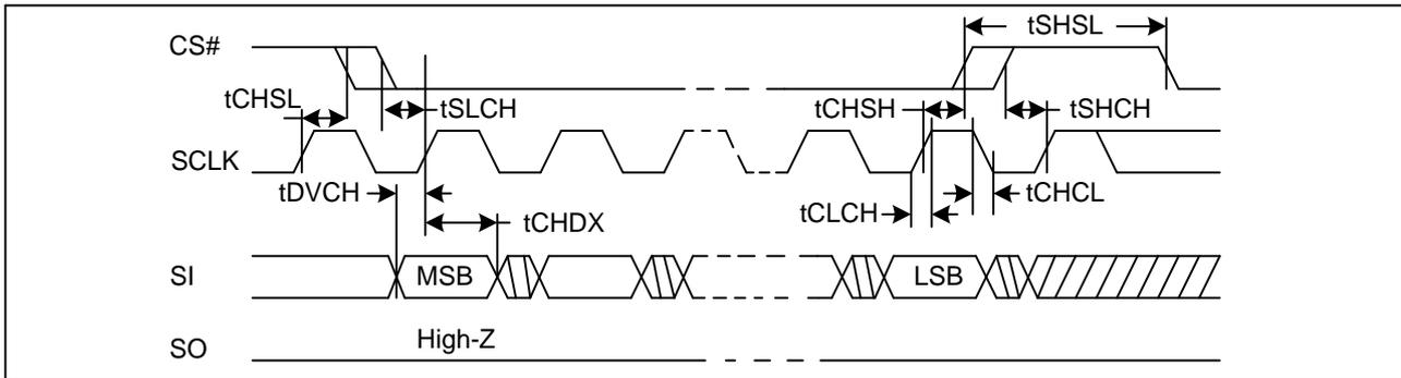
**Figure 41. Output Timing**
