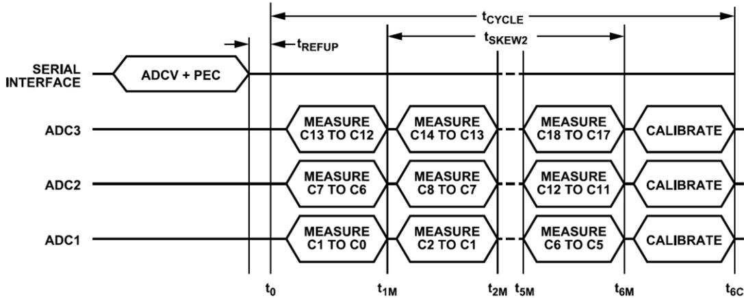
Figure 16. Timing for ADCV Command Measuring all 18 Cells
