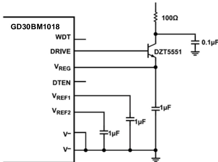
Figure 38. Simple VREG Power Source Using NPN Pass Transistor
