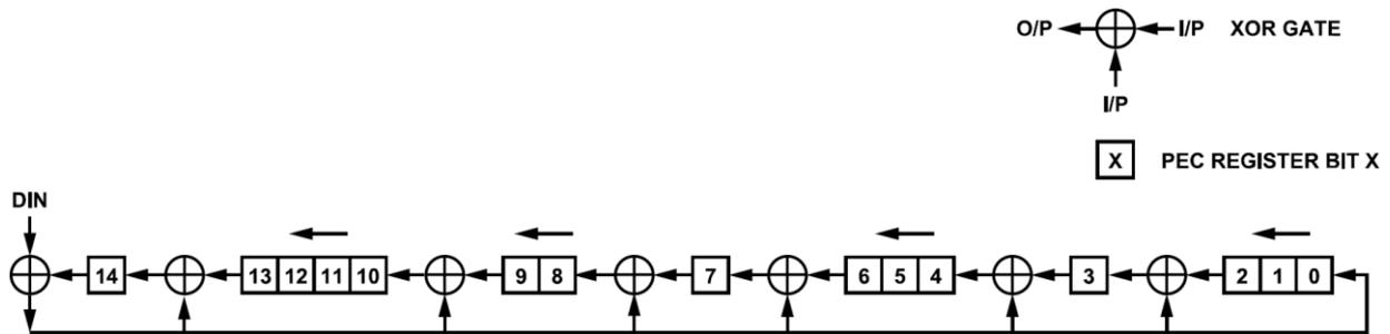
Figure 33. 15-Bit PEC Computation Circuit
