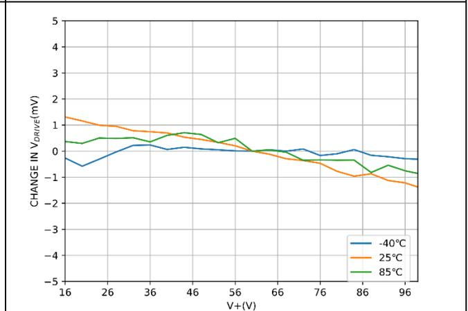
Figure 10. VDRIVE and V+ Line Regulation
