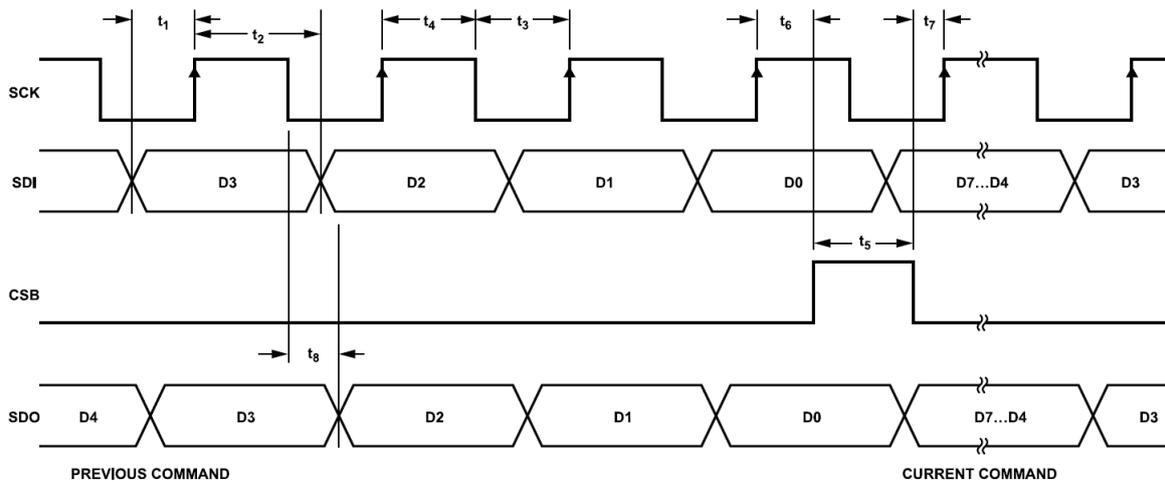
Figure 29. Timing Diagram of 4-Wire Serial Peripheral Interface
