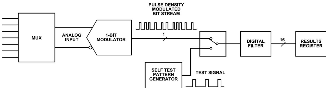
Figure 23. Operation of GD30BM1018 ADC Self Test
