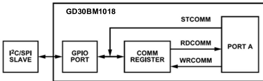
Figure 25. GD30BM1018 I2C or SPI Master Using GPIOs
