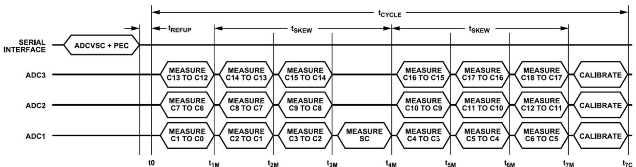
Figure 21. Timing of ADCVSC Command Measuring All 19 Cells, SC
