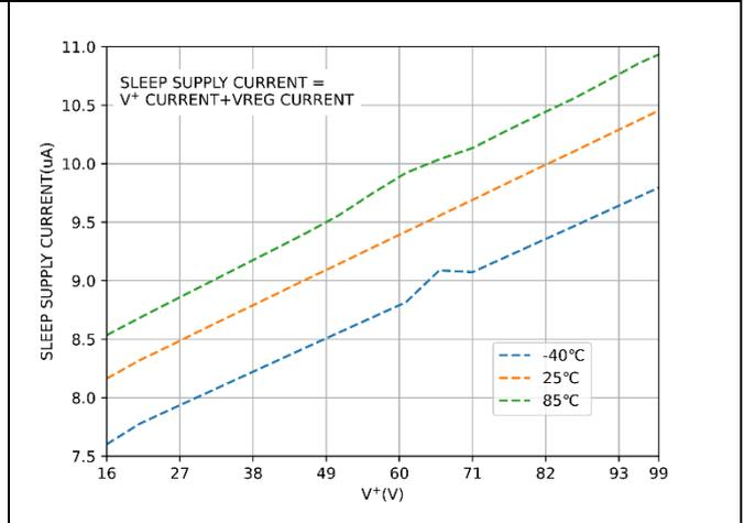
Figure 2. Sleep Supply Current vs. V+
