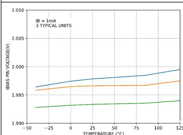
Figure 11. IBIAS Pin Voltage vs. Temperature
