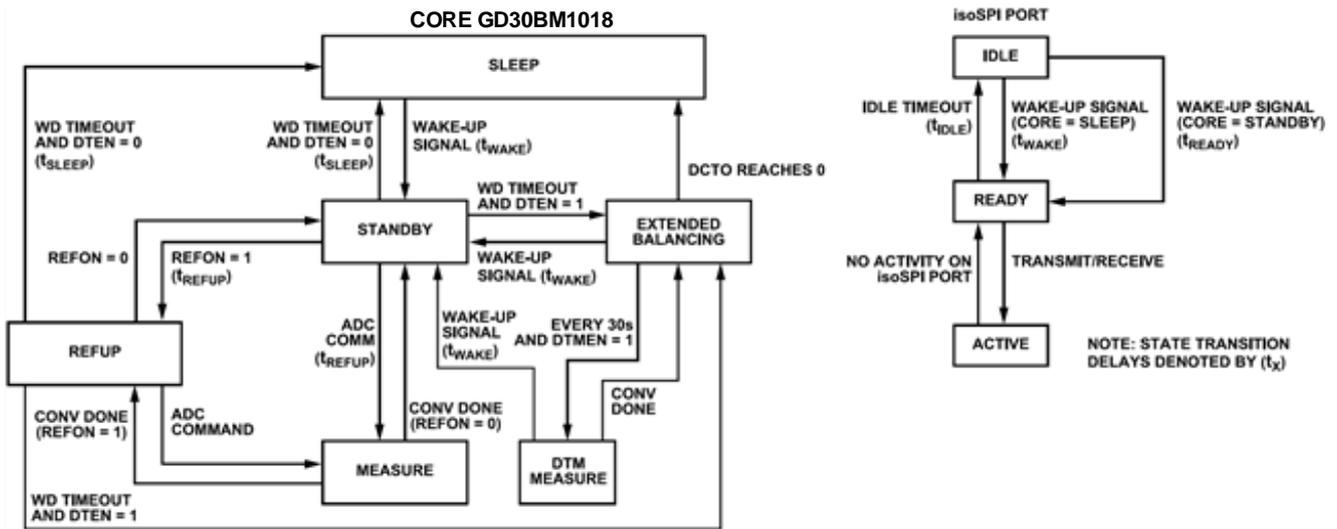
Figure 15. GD30BM1018 Operation State Diagram
