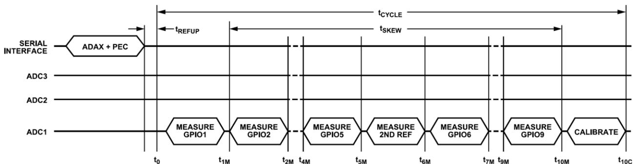
Figure 18. Timing for ADAX Command Measuring All GPIOs and 2nd Reference
