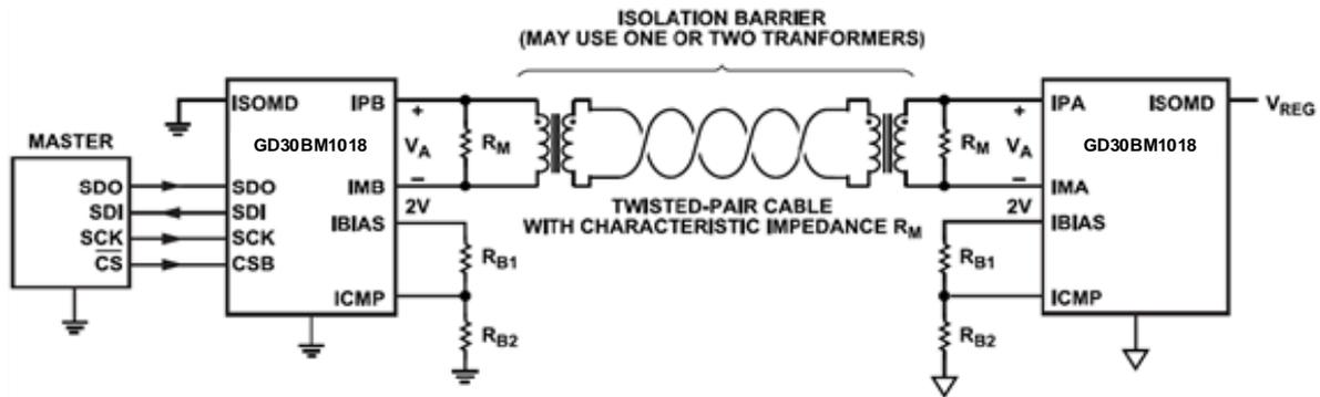
Figure 42. isoSPI Circuit
