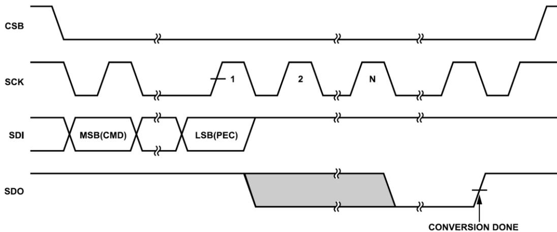
Figure 37. SDO Polling Using PLADC Command (Daisy-Chain Configuration)
