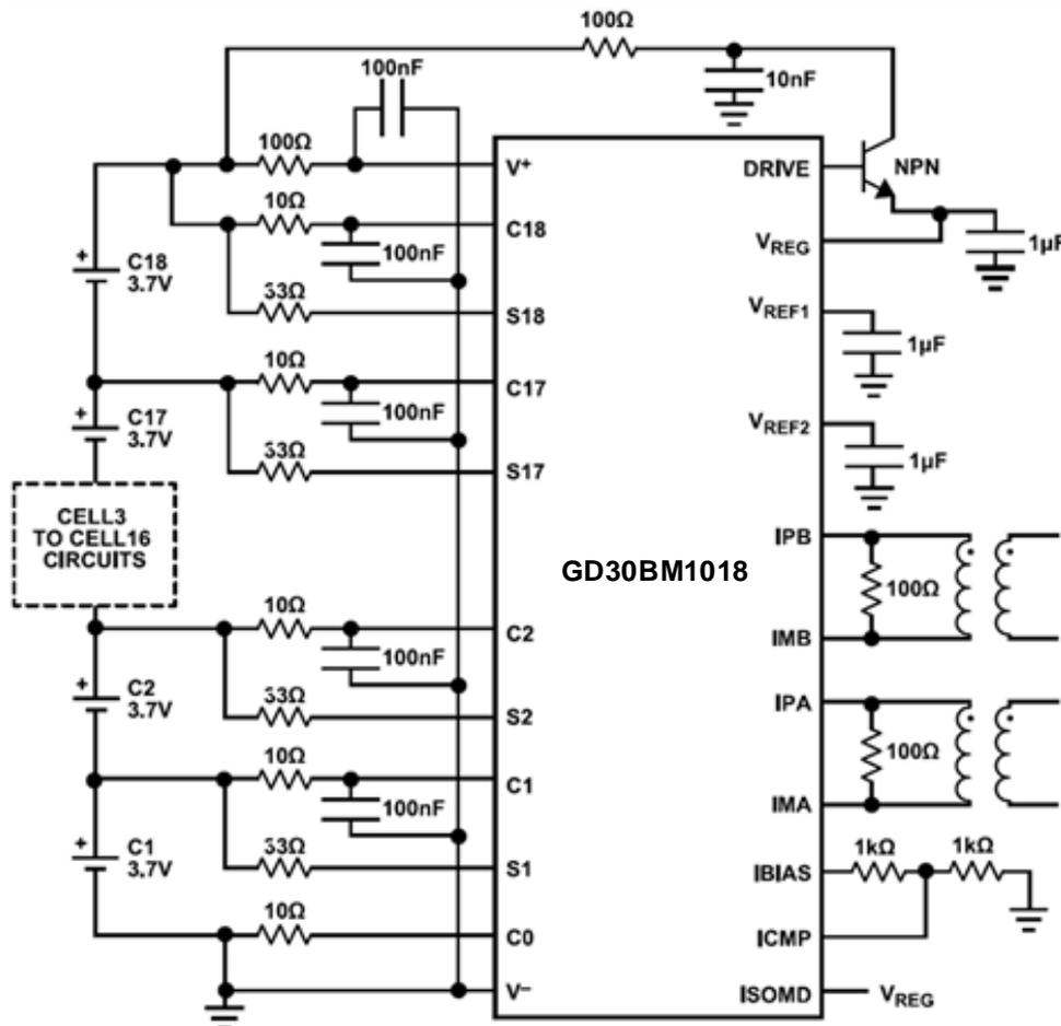
Figure 44. Schematic of GD30BM1018 Application
