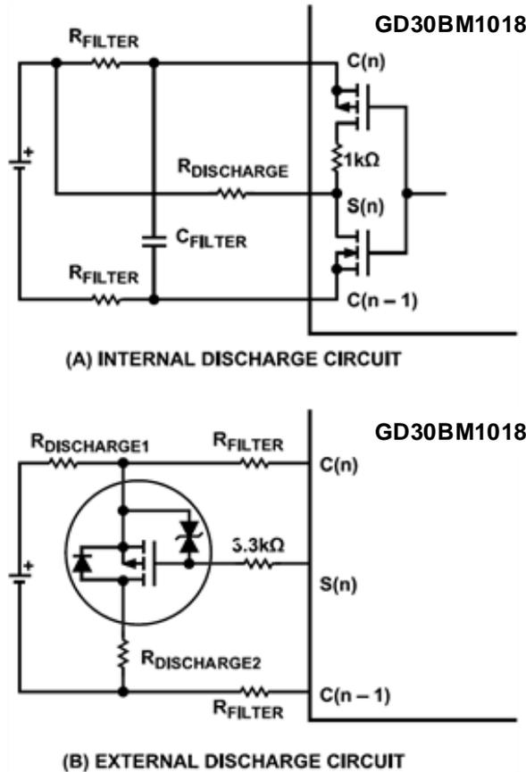
Figure 41. Balancing Self Test Circuit
