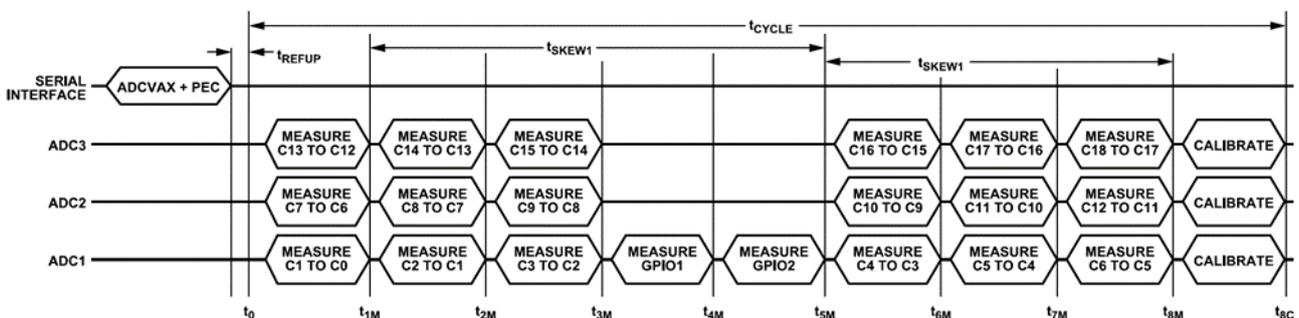
**Figure 19. Timing of ADCVAX Command**
