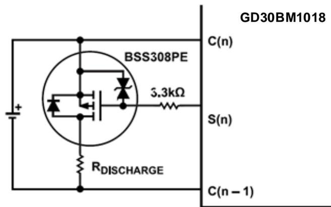
(B) EXTERNAL DISCHARGE CIRCUIT
