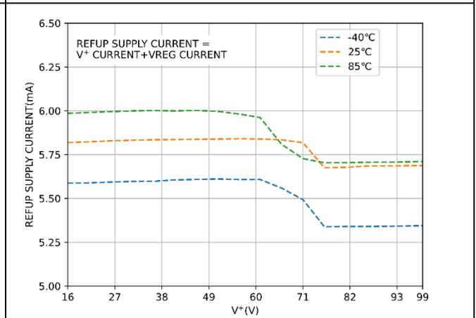
Figure 4. REFUP Supply Current vs. V+
