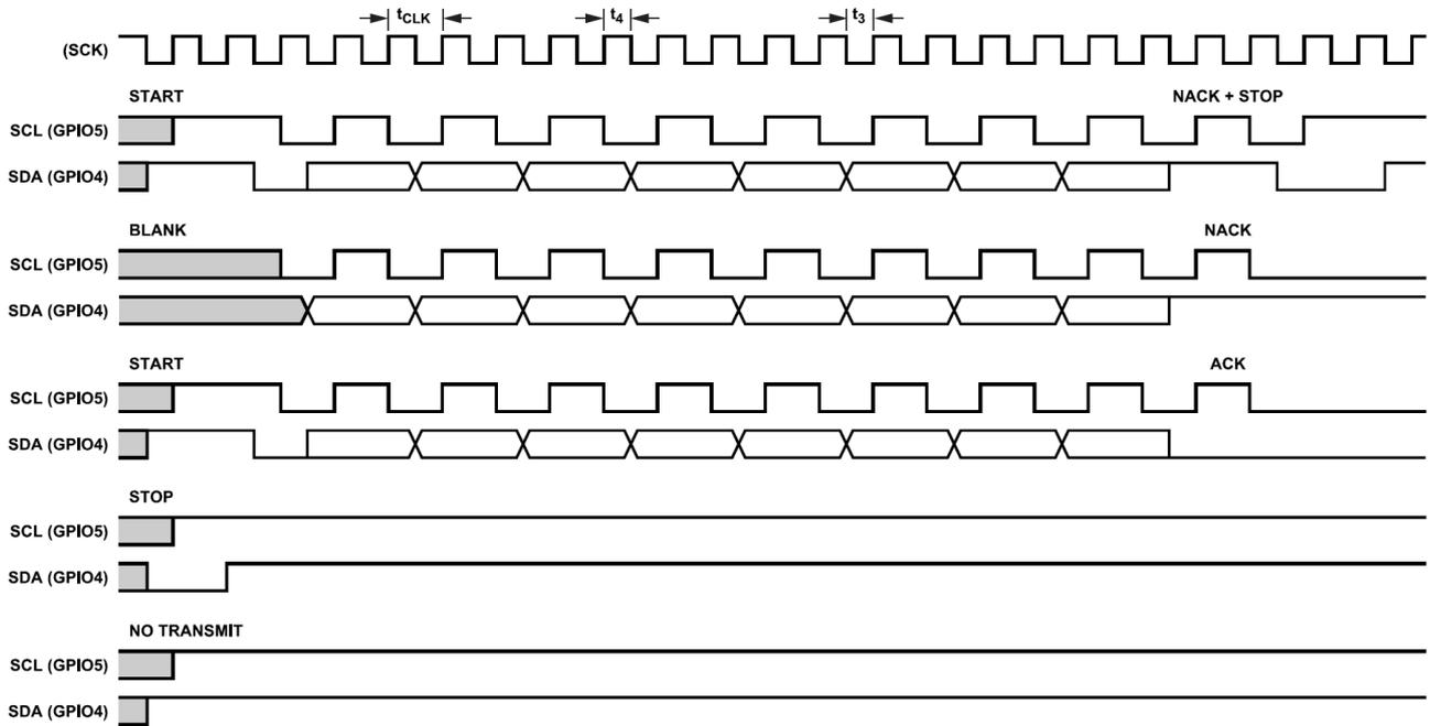
Figure 26. STCOMM Timing Diagram for an I2C Master
