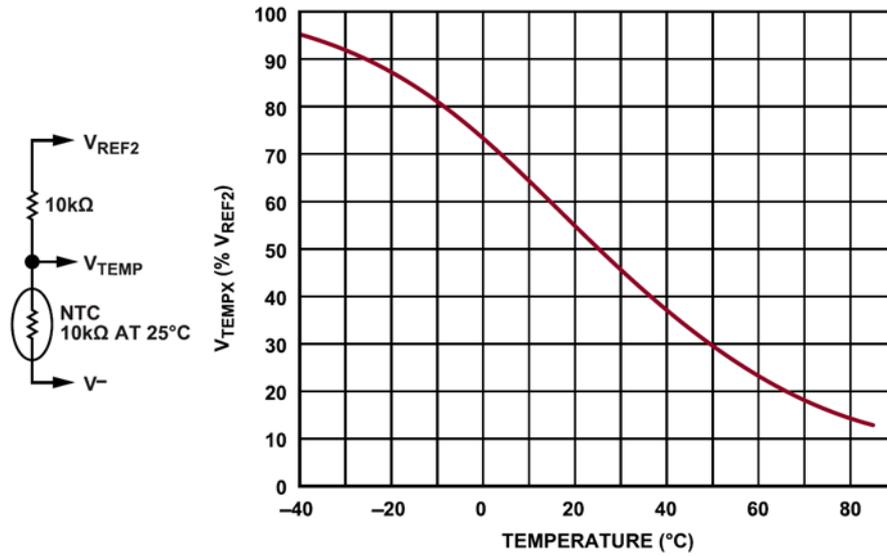
Figure 43. Typical Temperature Probe Circuit and Relative Output
