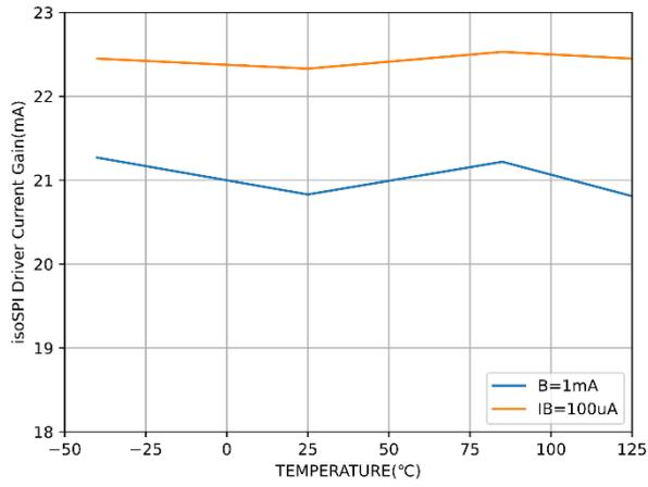
Figure 13. isoSPI Driver Current Gain(Port A and Port B) vs. Temperature
