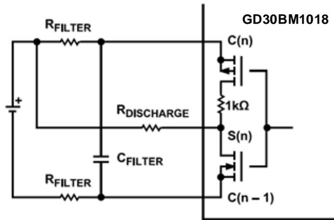
(A) INTERNAL DISCHARGE CIRCUIT
