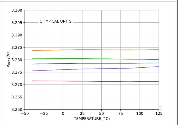
Figure 6. VREF1 vs. Temperature
