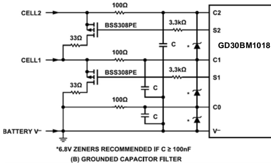
Figure 39. Input Filter Structure Configurations
