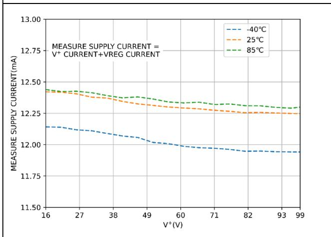
Figure 5. Measurement Supply Current vs. V+
