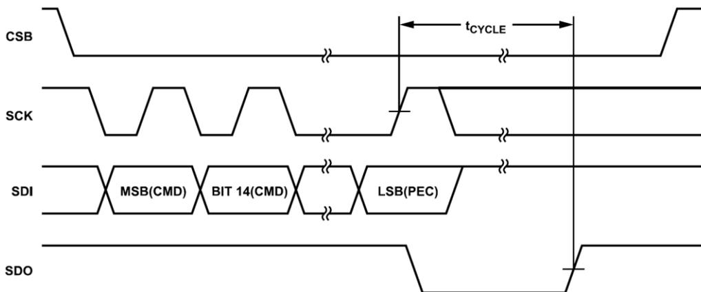
Figure 34. SDO Polling After an ADC Conversion Command (Single GD30BM1018)
