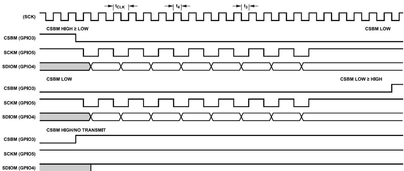
Figure 27. STCOMM Timing Diagram for an SPI Master
