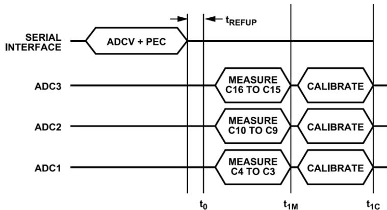
Figure 17. Timing for ADCV Command Measuring 3 Cells
