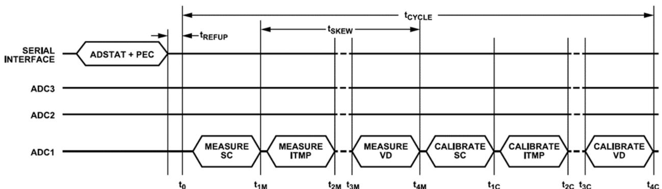
Figure 20. Timing for ADSTAT Command Measuring SC, ITMP, VA, and VD
