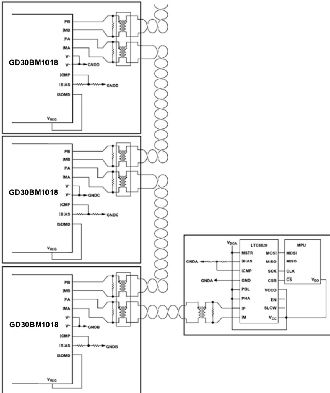
Figure 31. Transformer-Isolated Daisy-Chain Configuration
