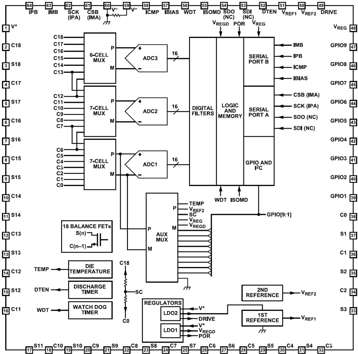
Figure 14. GD30BM1018 Functional Block Diagram
