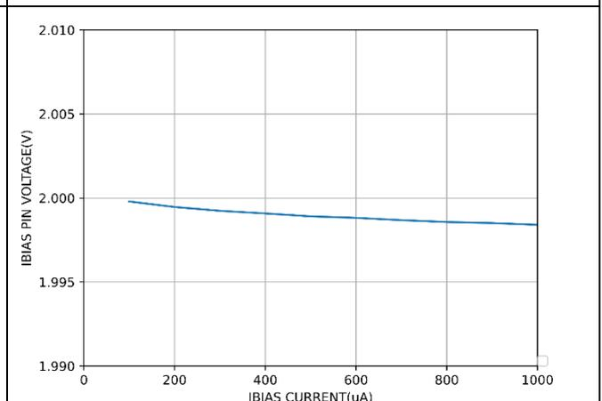
Figure 12. IBIAS Pin Voltage Load Regulation
