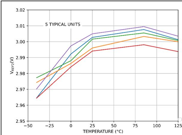
Figure 7. VREF2 vs. Temperature
