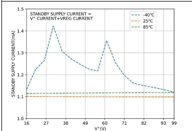
Figure 3. Standby Supply Current vs. V+
